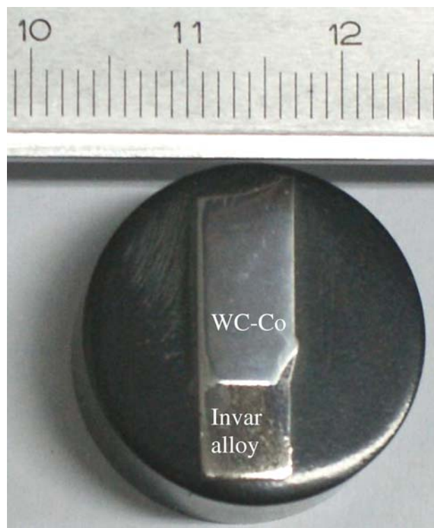
Fig. 2 Macro image of WC-Co/Invar weldment
